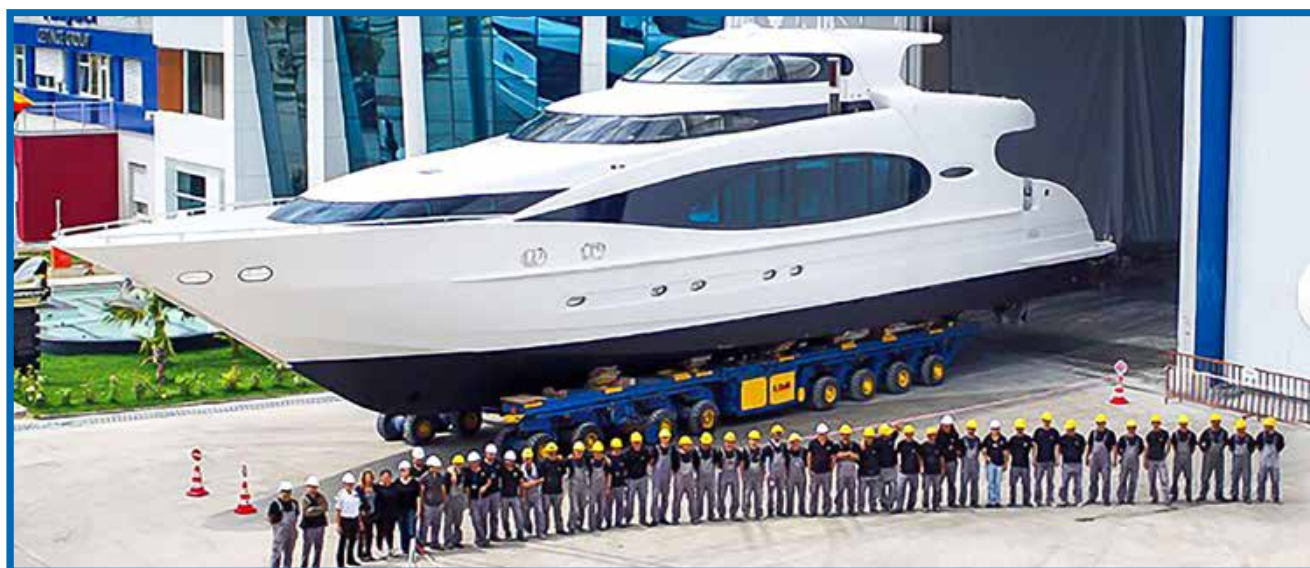
LIMASSOL (CYPRUS) - Limassol marina Mobile Boat Trailer - Capacity 40 t
