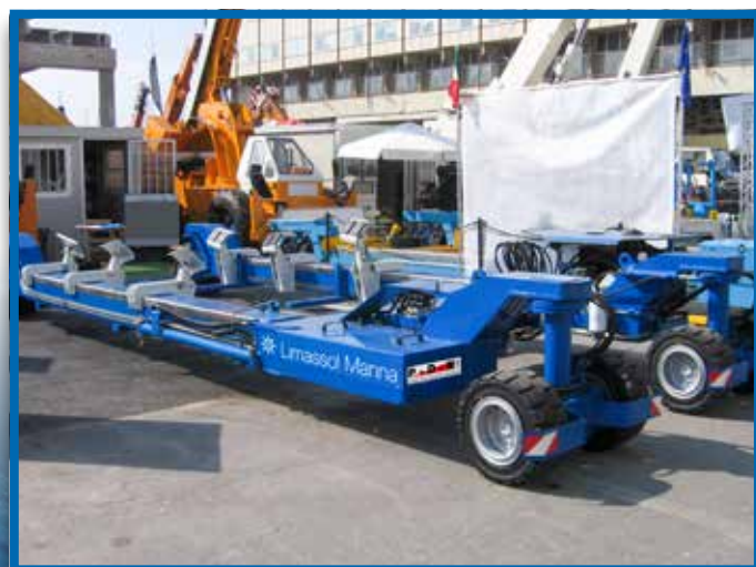
LIMASSOL (CYPRUS) - Limassol marina Mobile Boat Trailer - Capacity 40 t
